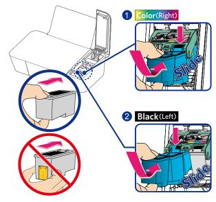
7 Set the Black Ink cartridge all the way into the slot on the left side.
