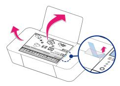
3 Open the Scanner lid, then remove the protective paper.
