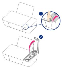
2 Press the Cartridge tab to open the Cartridge slot.
