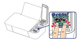
3 Remove the cartridges.
