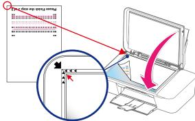
6 The unit will start scanning the alignment pattern to set an appropriate alignment on this unit.
