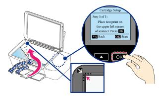
4 The unit will start scanning the alignment pattern to set an appropriate alignment on this unit.
