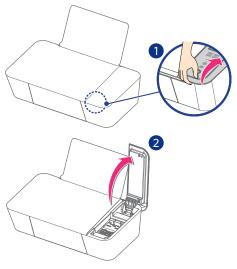
4 Press the Cartridge tab to open the cartridge slot.
