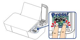
5 Set the color ink cartridge all the way into the cartridge slot on the right side.
