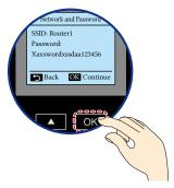
5 [Connected to ...] message will appear on the Menu display when the Connection is successful. Press ok twice, then the Connection setting is completed.
