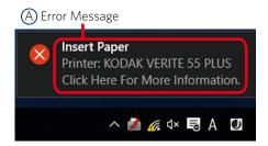
A pop-up appears from the system tray icon to provide immediate error notification. If you click on the pop-up, an error recovery guide appears so that you can confirm a detailed explanation on how to fix the problem.
